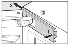
■ Remove cover <sup>③</sup> from the inside of the bearing block and slide it out.
